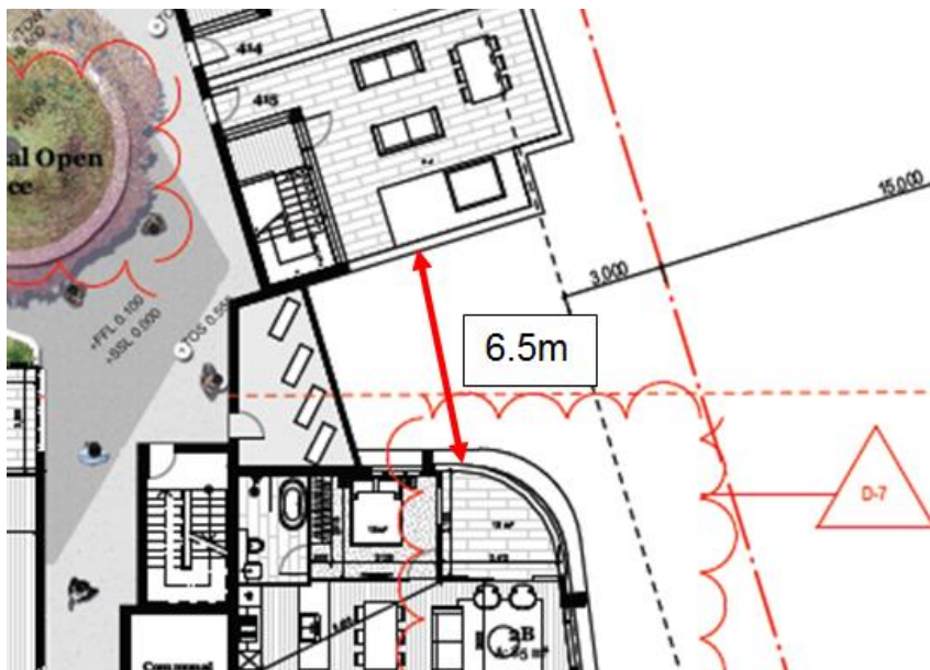
Figure 18: Separation distance between balconies – L6
